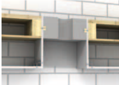
Wooden beam ceiling with classified ceiling substructure
